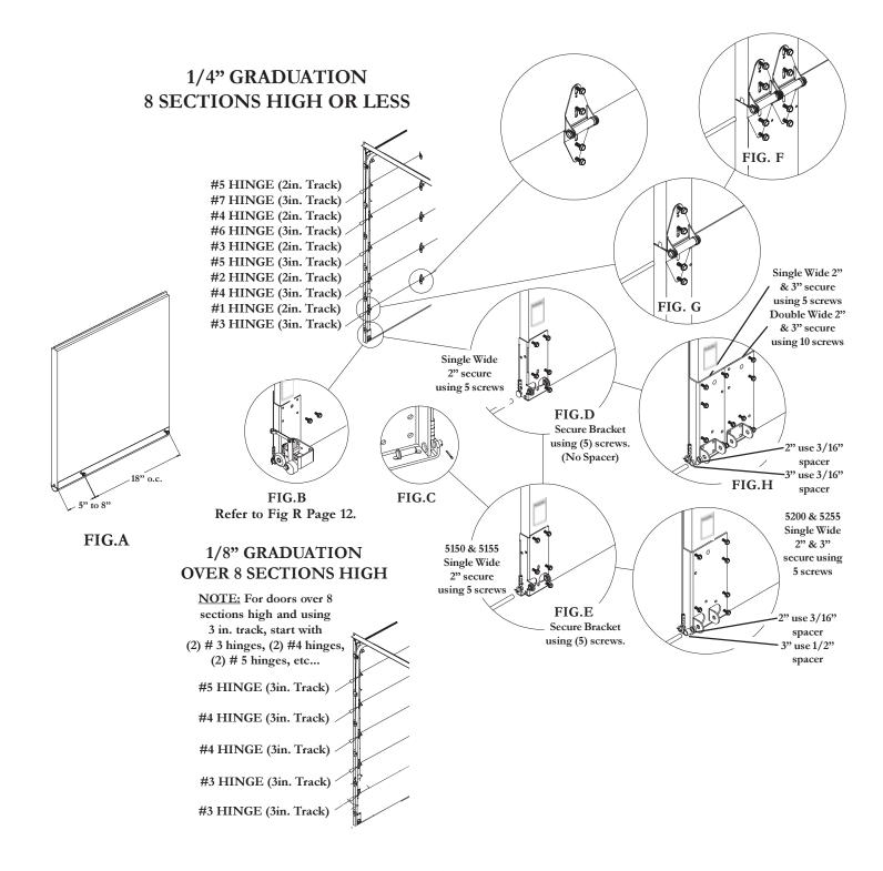
STEP 3. Locate the bottom section, attach bottom seal using 1/4" self drilling and tapping screws as shown in Fig. A.
